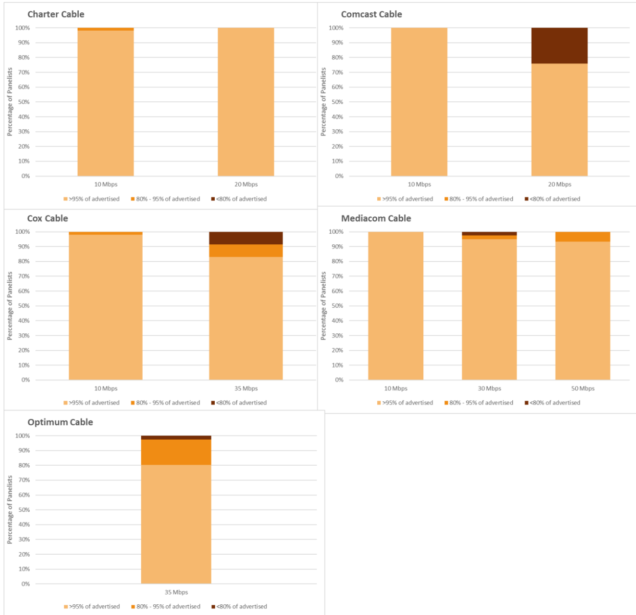
Chart 20.2: The percentage of consumers whose median upload speed was greater than 95%, between 80% and 95%, or less than 80% of the advertised upload speed (cable).
